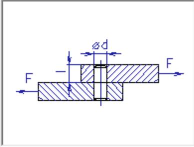
The diagram shows a cross-section of a cylindrical pin of diameter  $d$  passing through two plates. A shear force  $F$  is applied to the plates, causing them to slide relative to each other. The pin is shown in a shaded state, indicating it is under stress.
